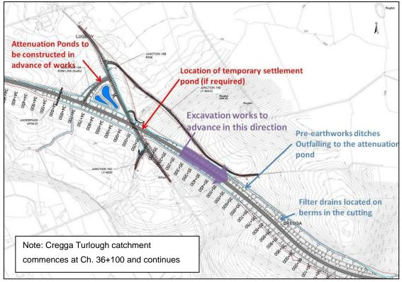
Plate 7.1 Construction Sequencing Between Ch. 35+150 and 36+450
