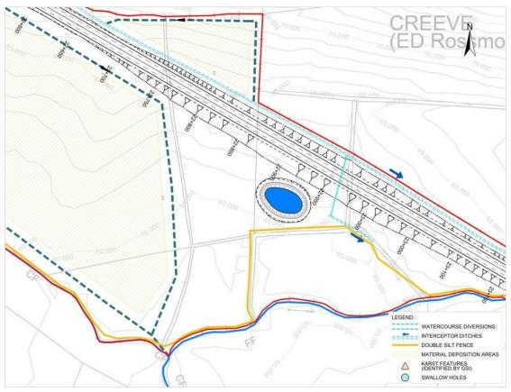
Plate A1.7 – Attenuation Pond Located at Ch.23+200
