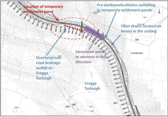
Plate 7.2 Construction Sequencing Between Ch. 36+900 to Ch. 37+650
